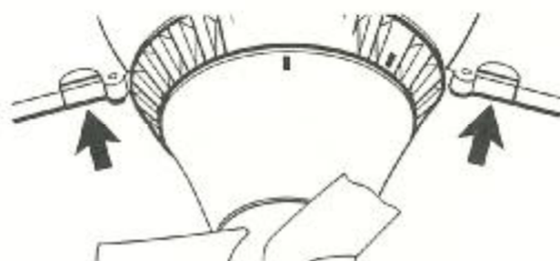
Check that the clamp lock levers do not stick out.
