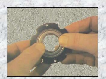
The large bearing and housing are now fitted to the shaft. The housing flange side (wide diameter) facing down.
