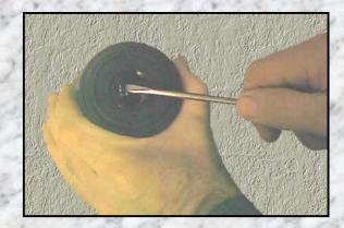
Using a screw driver or suitable probe prise up the FA seal, remove and discard.
