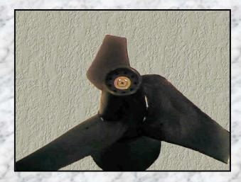
Remove pitch adjusting knob screw. (counterclockwise)
