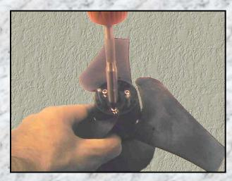
Lift the blade retainer from the casing.
