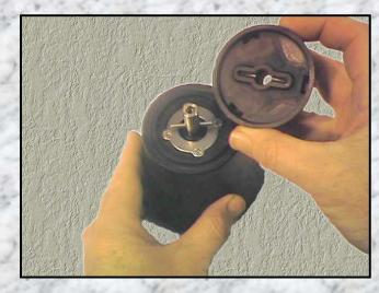
The clutch screw assembly is now fitted. The star washer sits on the boss first, next the spring cup washer, the inner edge should sit on the star washer and the outer edge is curved up.
