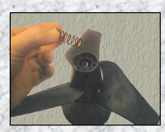
Lift the pitch adjusting knob from the propeller blades.
