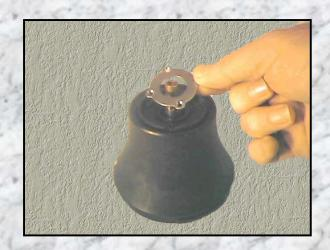
Use an o ring pick, taking care not to score the sealing surface, remove the seal retainer o ring from around the outer edge of the seal. Discard this o ring it is to be replaced after each removal.
