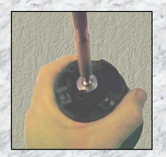
Lubricate the blade locating slots in the boss with silicone grease. A heavy lube is required.
