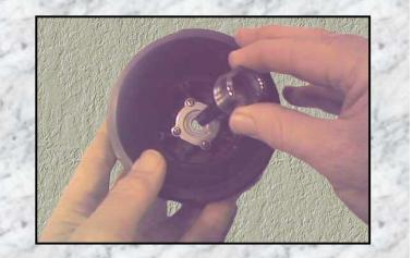
The large bearing is now pressed by hand into the bearing housing.
