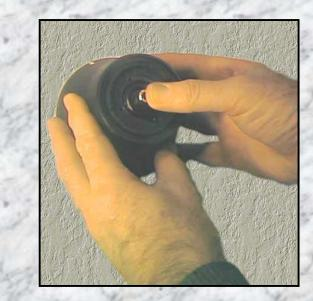
The bearing, propeller shaft and bearing housing can be removed as a unit.
