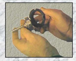
After removing the large 'C' ring from the propeller shaft support the bearing by the inner race in a suitable vice, using a nylon rod and small hammer,gently tap the shaft through the bearing.
