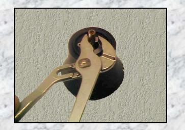
Turn the housing over to gain access to the four screws that secure the large bearing housing. Remove these screws and washers.
