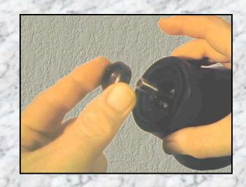
Press the seal gently around the edges until it is flush in the casing.
